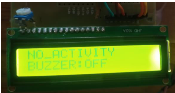
Fig(C): "No Activity Detected": Buzzer Remains Off, Indicating Normal Conditions.
